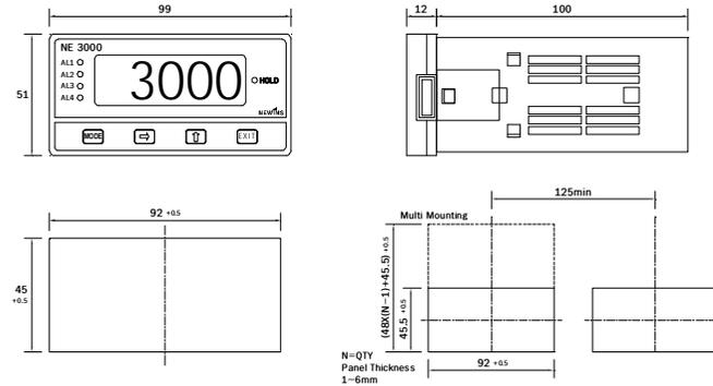
**△ Caution :** Maintenance and to ensure the safety of the device if you add a space to more than 125mm size is recommended.
